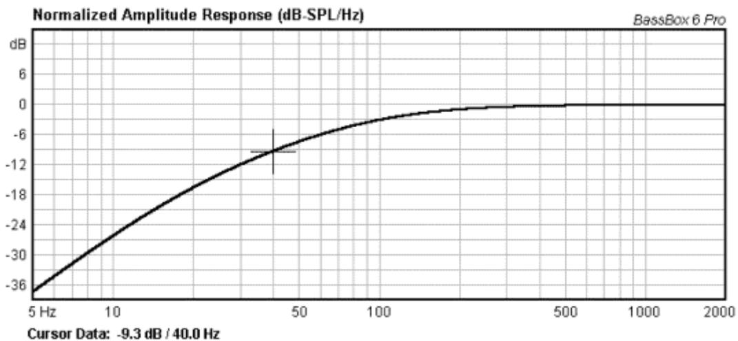
From the graph we see that it is necessary to boost by about 14 dB at 25 Hz with a low pass slope of 12 dB/oct. to achieve a flat response.
