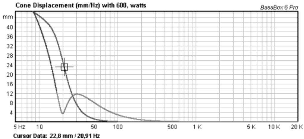
The cone displacement of both the passive and active driver is OK within the safe operating limits of the drivers. However it can be seen that the cone displacement rises steeply below 20Hz meaning that a high pass filter to protect against overload is highly recommended.
