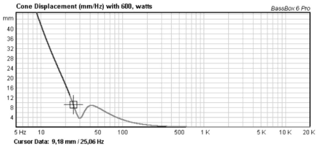
In the 12" case the first maximum appears around 38-40 Hz. From the graph it can be seen that the design is safe in this region reaching about +/- 9,2mm.
