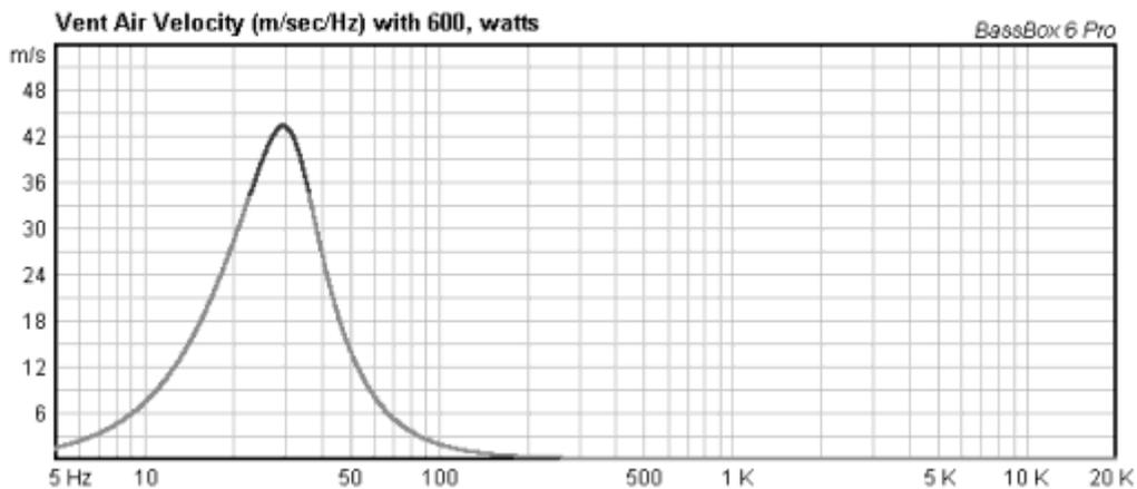
This means that a larger diameter of port is needed, which will require that the port is longer. Using a  $\varnothing 90$  mm port and 510 mm of length turns out to be a good choice:
