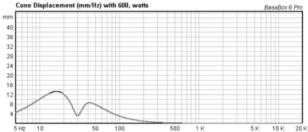
The first peak is the same around 9,2 mm but the uncontrolled rise in displacement below tuning is now controlled so that the maximum is reached at about 17 Hz and is below 14 mm. It should be clear to everyone that the high pass filter is a great improvement especially considering that the system is not able to produce any SPL below 20 Hz anyway.
