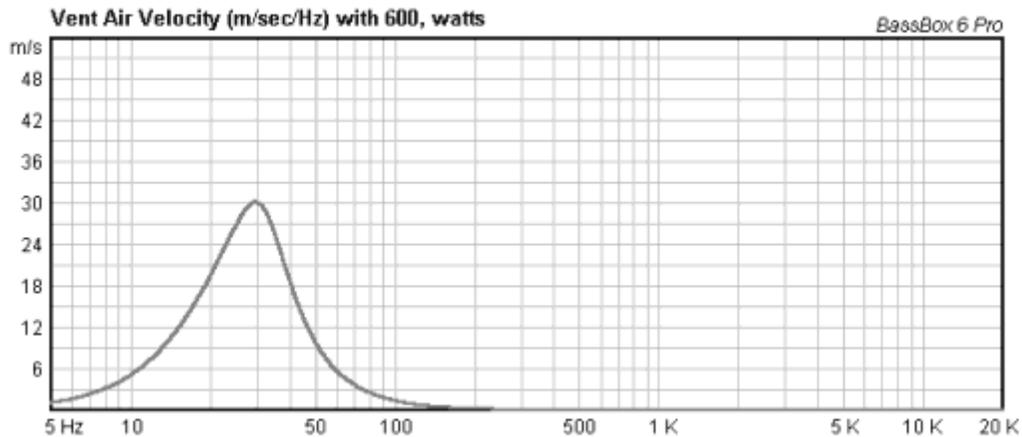
Now the velocity is below 35 m/s and if a double flared port is chosen a good result should be possible.
