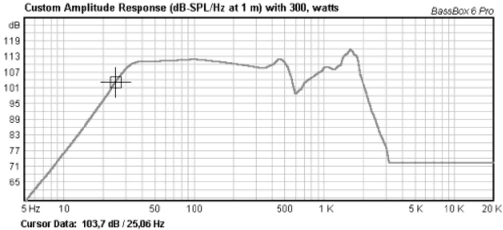
From the simulation it can be seen that the system response is up by about 3 dB at 25 Hz compared to the sealed box. We get about 104 dB with 300 W RMS at 25 Hz.
