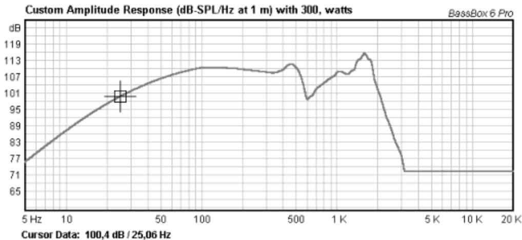
From the graph we see that it is necessary to boost by about 10 dB at 25 Hz with a low pass slope of 12 dB/oct. to achieve a flat response.
